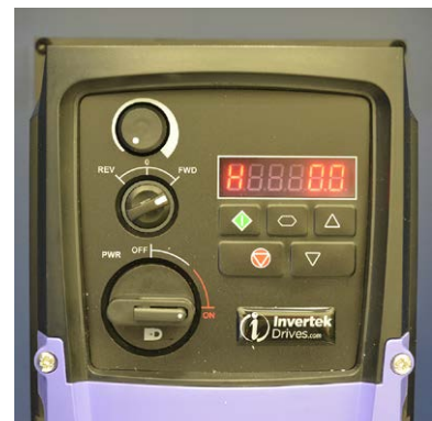
Fig. 8c Switch 2 set to FWD
